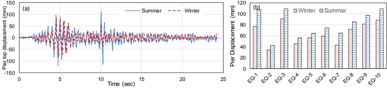
Figure 5. (a) Pier top displacement-time history of the isolated bridge under EQ#10, (b) Pier top displacement comparison under summer and winter condition
