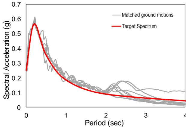
Figure 3. Scaled response spectra of the selected records
