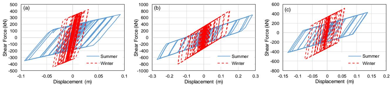
Figure 8. Hysteretic response of LRBs under summer and winter (a) Long pier, (b) Short pier, and (c) Medium pier
