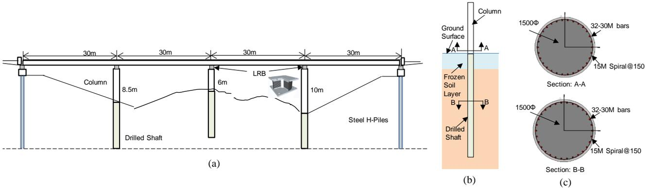
Figure 1. (a) Elevation of the bridge studied, (b) Details of the soil-foundation system, (c) cross section of column and drilled shaft
