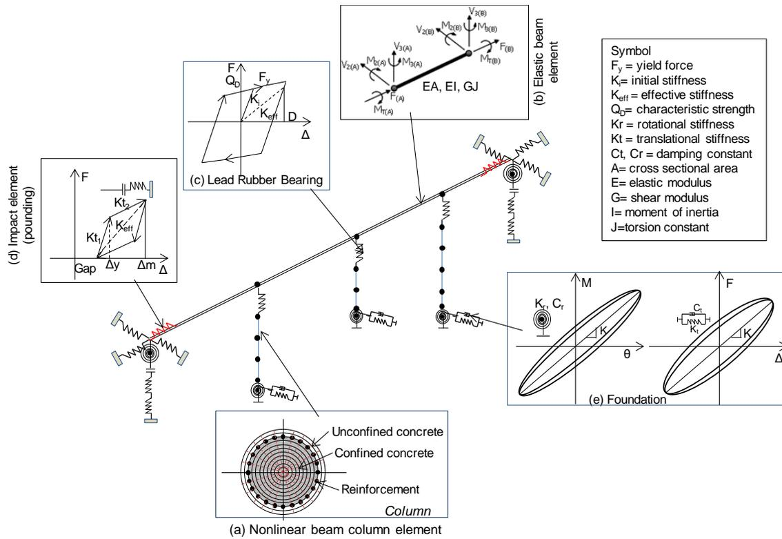
Figure 2. Details of the finite element model of the bridge
