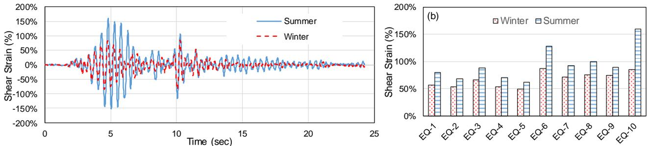
Figure 7. (a) LRB shear strain-time history of the isolated bridge under EQ#10, (b) LRB shear strain comparison under summer and winter condition
