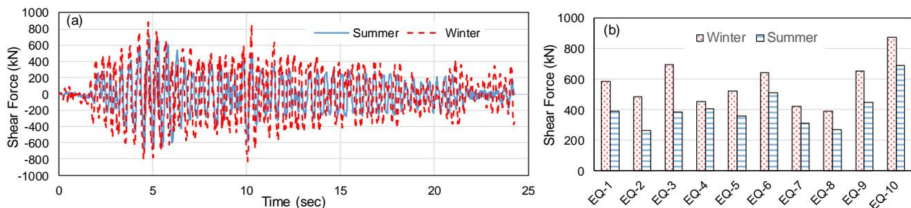
Figure 4. (a) Base shear-time history of the isolated bridge under EQ#10, (b) Shear force comparison under summer and winter condition
