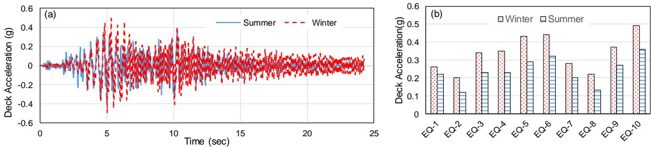
Figure 6. (a) Deck acceleration-time history of the isolated bridge under EQ#10, (b) Deck acceleration comparison under summer and winter condition
